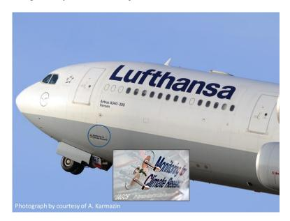
Figure 2. IAGOS-CORE installation position aboard the Lufthansa A340-300 "Viersen" (photograph by courtesy of A. Karmazin); the insert shows details of the IAGOS Inlet Plate which carries the inlet probes for trace gas sampling (photograph by courtesy of Lufthansa).
